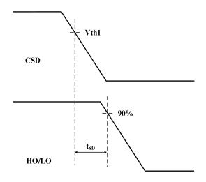
Figure 8-1. Switching Time Waveform Definitions
