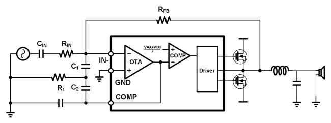
Figure 10-3 Typical Control Loop Design
