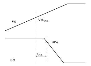
Figure 8-3. VS > VthOCL to Shutdown Waveform
