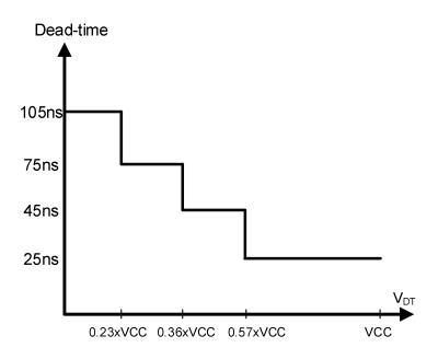
Figure10-6 Dead Time vs. V<sub>DT</sub>
