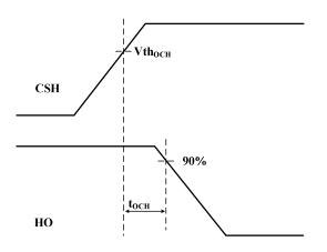
Figure 8-4. VCSH > VthOCH to Shutdown Waveform
